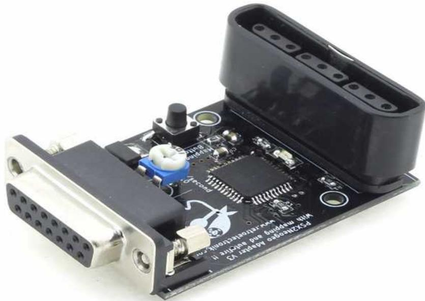
*Retroelectronik PSX2NeoGeo pad adapter V2*
